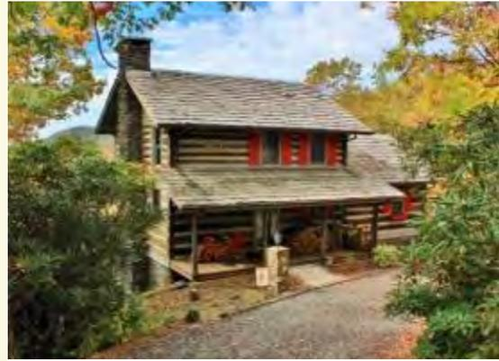
The initial coating on the home required about 7 gallons. To avoid staining the chinking, the product was painted on using a 3-inch width natural bristle brush. Sufficient material was painted on each log to the point of "saturation" as evidenced by no further absorption.
